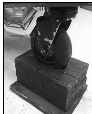
Wood block with caster groove cut out (6" x 3" x 4" = Width x Depth x Height):
