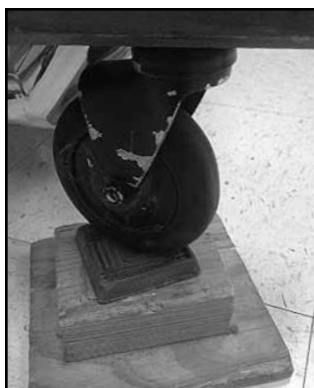
Wood block with rubber gasket on top (4" x 4" x 2"):
